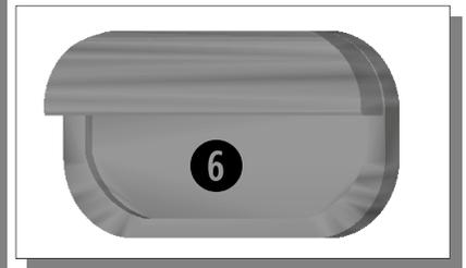
**End is cut away and part of bottom panel is removed to reveal support structure.**
